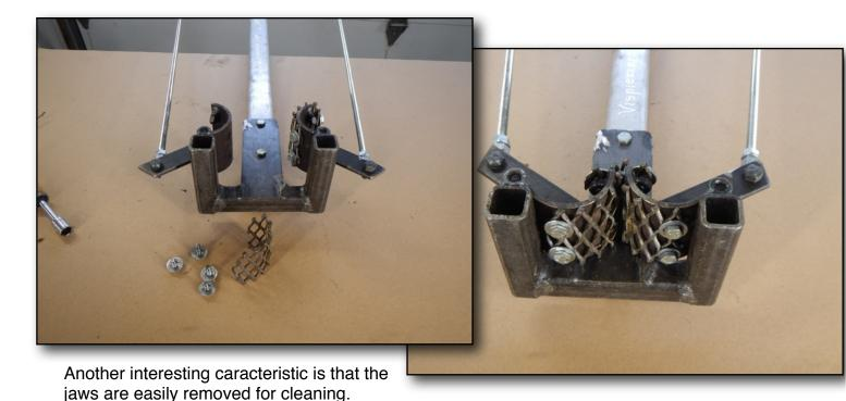
The SMART is to be assembled with a piece wood (2 X 2) purchased by the buyer to connect the handles with the jaws. It also needs to have 5/16th threaded rods to operate the jaws. It is supplied with guides on the base and also on the handles to install the piece of wood. It can be ordered with an aluminum tubing instead of wood which gives a professional look.
